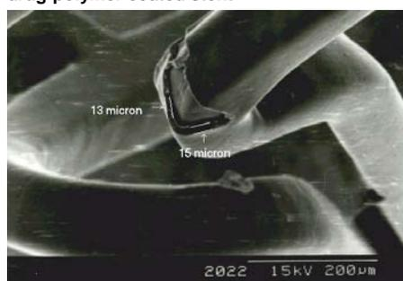
Fig. 8: SEM micrograph showing coating thickness on stent surface at two different locations
