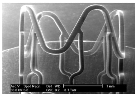
Fig. 7: SEM micrograph showing dilation profile of drug-polymer coated stent
