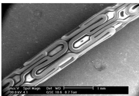
Fig. 6: Scanning electron micrograph showing crimping profile of drug-polymer coated stent
