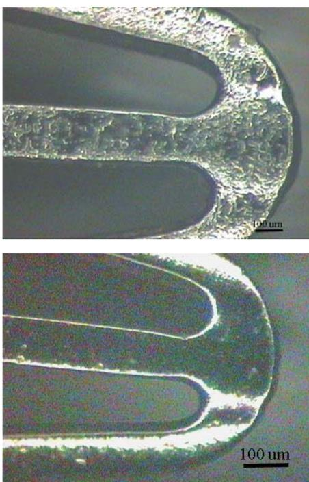
Fig. 3: Optical micrographs showing effect of atomization pressure on surface smoothness of coated stent.
