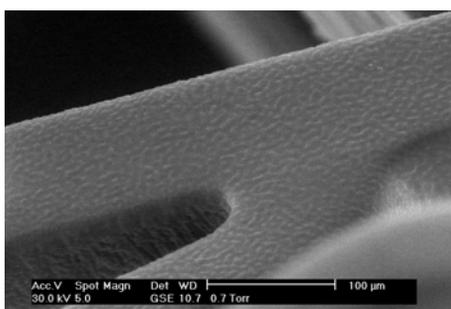
Fig. 5: SEM micrograph illustrating typical morphology of drug-polymer coated stent surface.
