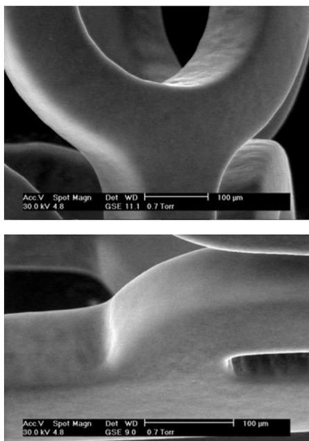
Fig. 4: SEM micrograph showing drug-polymer coated stent
