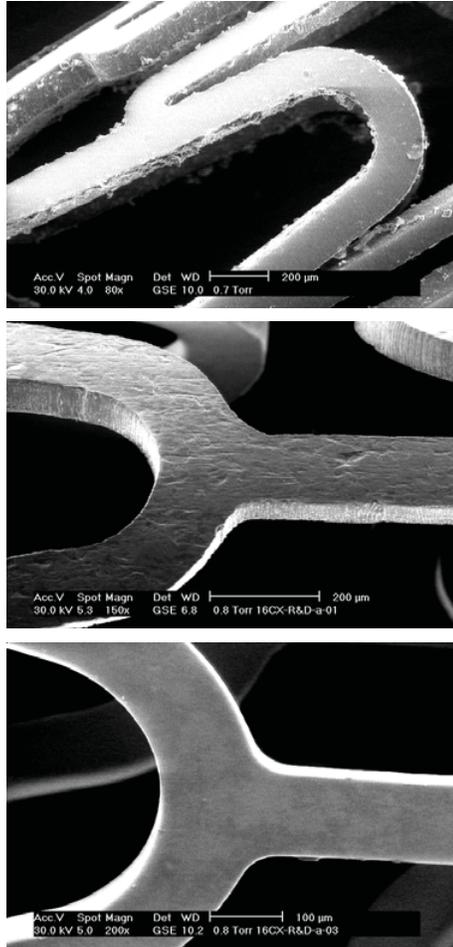
Figure 4: SEM images of (a) Laser cut stent, (b) pickled stent, (c) electropolished stent
