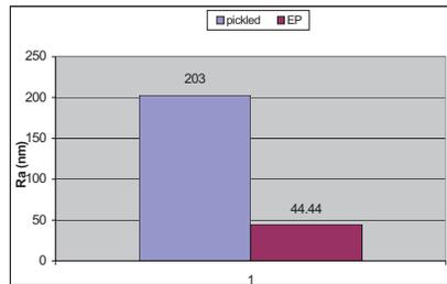
Figure 6: Plot for roughness comparison (5μ area)
