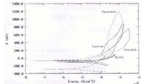
**Figure 9: Cyclic polarization test for pitting potential evaluation**
