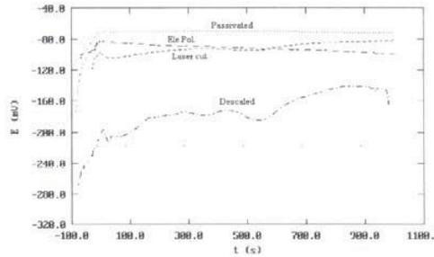
**Figure 7: Corrosion Potential Stabilization Curve**
