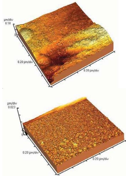
Figure 5: High-resolution AFM images of stents (a) Acid pickled stent (b) electropolished stent
