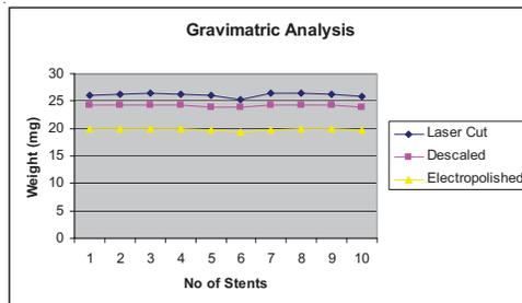
**Figure 2: Plot showing variation in stent weight**
