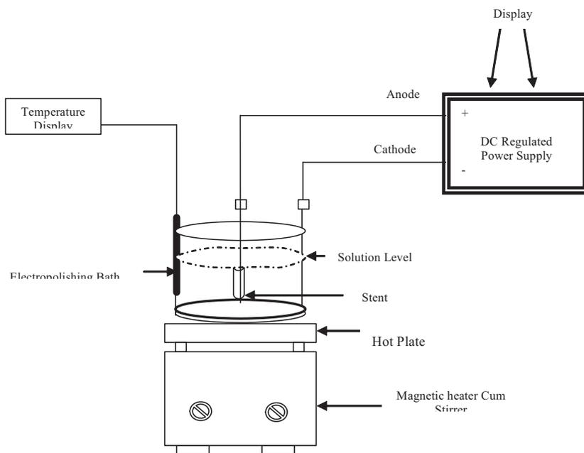
**Figure 1: Schematic of electropolishing setup**
