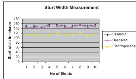
**Figure 3: Plot showing variation in stent width**
