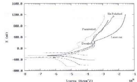
**Figure 8: Potentiodynamic test curves for passivity and Corrosion rates**
