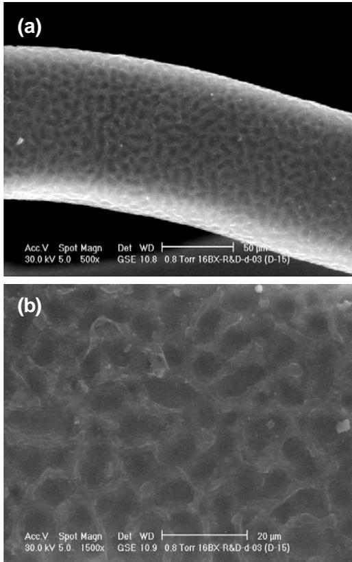
**Fig 4: (a) & (b): Scanning Electron Micrograph of drug-polymer coated stent after incubating in PBS at 37°C for 15 days**
