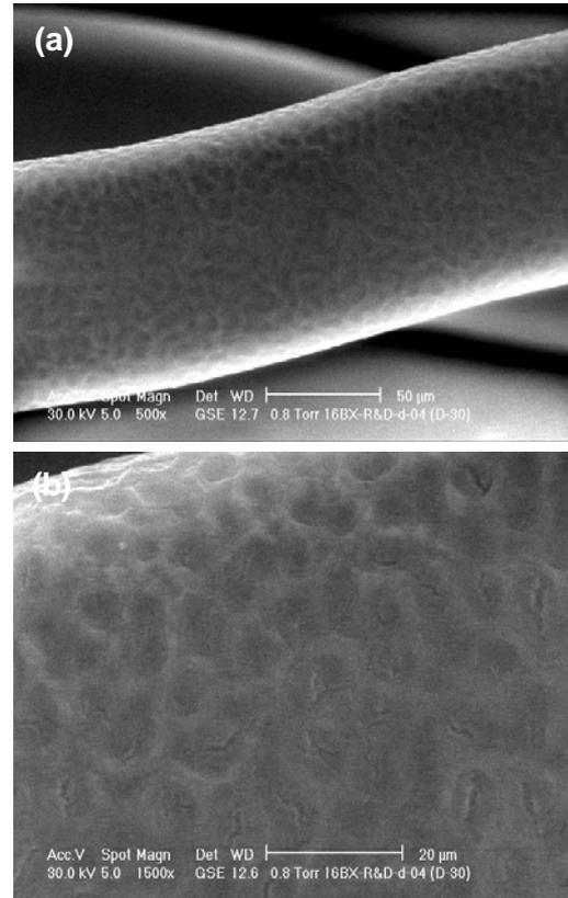
**Fig 5: (a) & (b): Scanning Electron Micrograph of drug-polymer coated stent after incubating in PBS at 37°C for 30 days**
