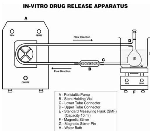
**Fig 1: Commercial apparatus for continuous flow method using peristaltic pump with recirculating buffer solution**
