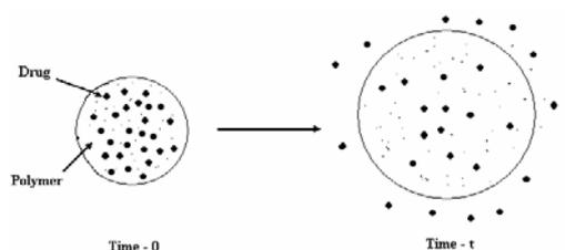
Fig 2: Schematic representation of drug release form drug-polymer matrix
