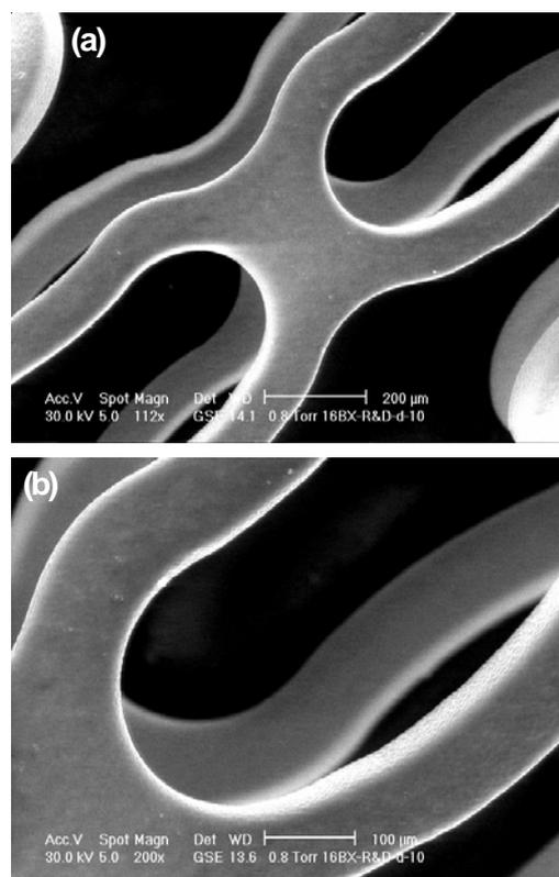
Fig 3: (a) & (b): Scanning Electron Micrograph of drug-polymer coated stent
